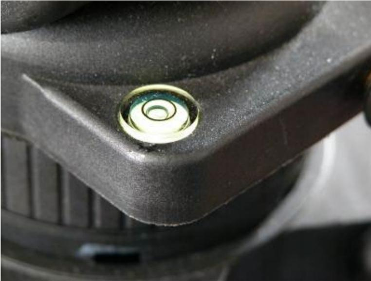
**Bubble level as part of the tripod head**
